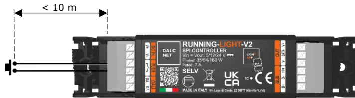
Figure 9: Local Control wiring diagram for Short Distances
