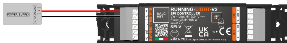
Figure 15: Power Supply wiring Diagram
